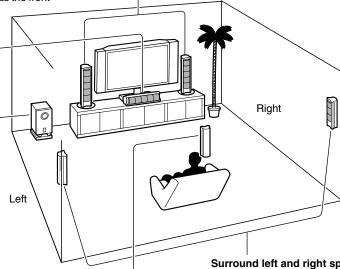
The subwoofer handles the bass sounds of the LFE (Low-Frequency Effects) channel. The volume and quality of the bass output from your subwoofer will depend on its position, the shape of your listening room, and your listening position. In general, a good bass sound can be obtained by installing the subwoofer in a front corner, or at one-third the width of the wall, as shown.
